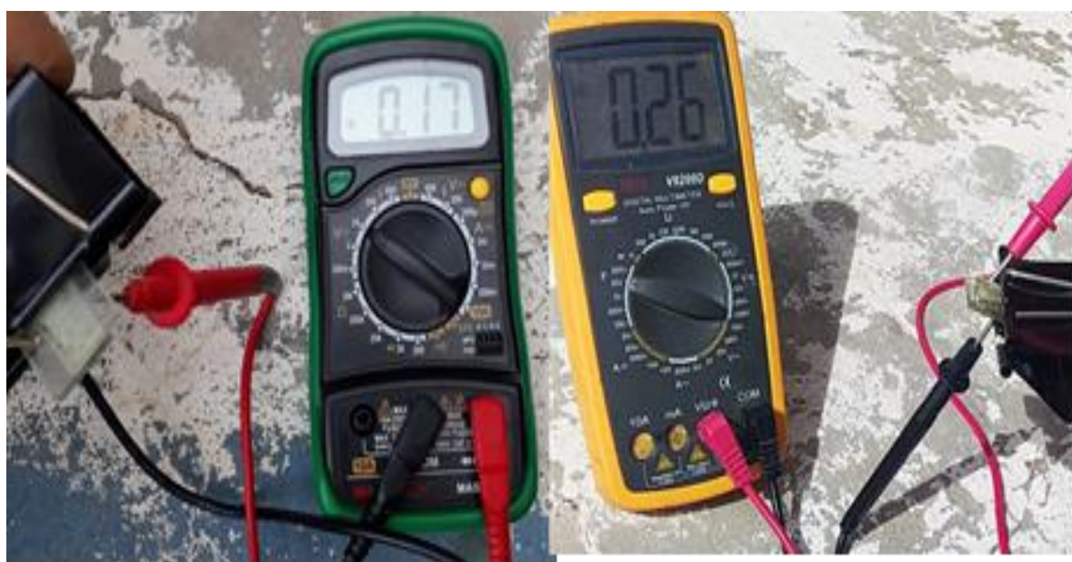
Figure 3. Voltage and Capacitance readings of carrot dye
