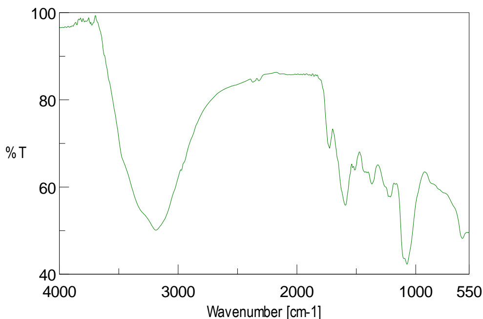
Figure 7. FTIR Spectrum of Cu nanoparticles prepared from Pepper Seed extract
